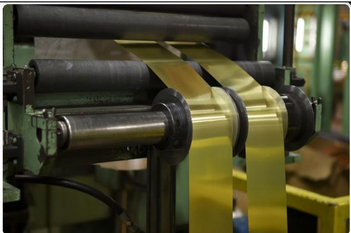
Reading Eagle: Lauren A. Little | Material comes off the slitting machine.
